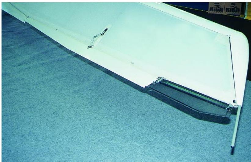
DHV-certificated Class 2 Stalker, with ailerons and tip draggers
