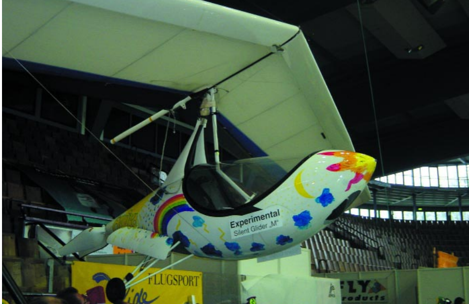
Experimental ultralight motor glider from Aeros, complete with folding prop, retractable undercarriage and strange control system
